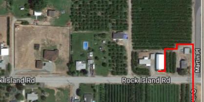
Effluent from individual septic tanks is pumped uphill, and into 6 dosing tanks located on Rock Island Road.
