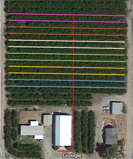
Perforated piping then distributes waste underground in drainage fields. A drainage field is composed of 2 rows of the cherry orchard and is designed to handle as much as 3,240 gallons of effluent per day. Control panels for pumps, float switches, and alarm system for the 6 dosing tanks on Rock Island Road.
